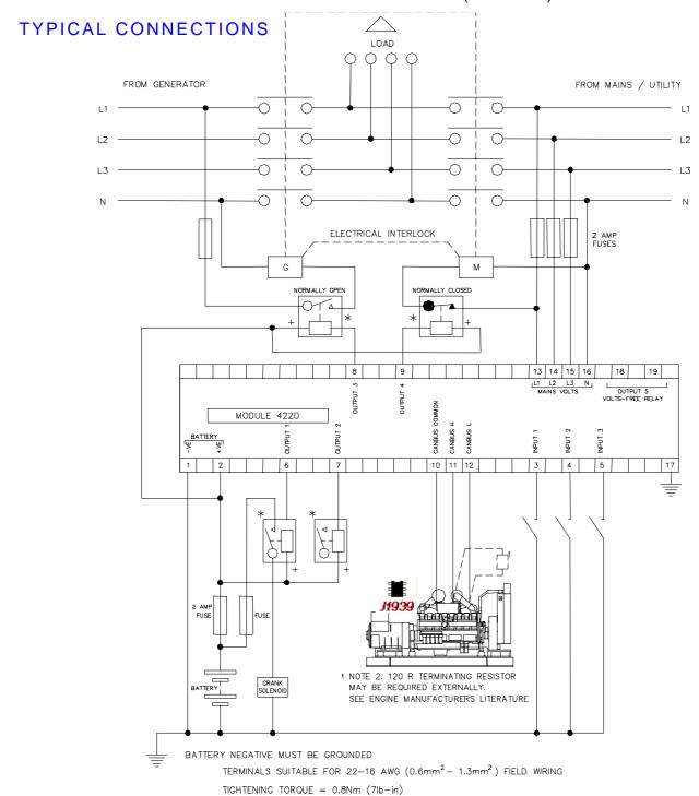
\* NOTE. SOME OF THE OUTPUTS ARE SOLID STATE AND ARE NEGATIVE SWITCHING
