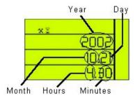
To edit the time, press the  $\checkmark$  button. The time, 4.30 in this example, will begin flashing. Press the + or - buttons to adjust the time in one minute steps until the desired time is shown. Press the  $\checkmark$  button to save the change. The time stops flashing to confirm that it has been successfully stored. Example: This display is showing a time of 4:30 on  $21^{st}$  October 2002.
